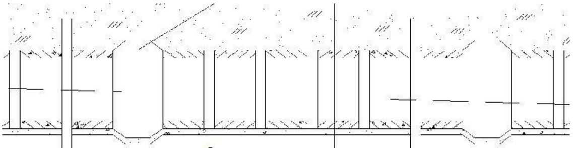
Figure 7 Pipeline unit Energy dissipation chamber is a hydrotechnical construction, which reduces the speed of water currents.
