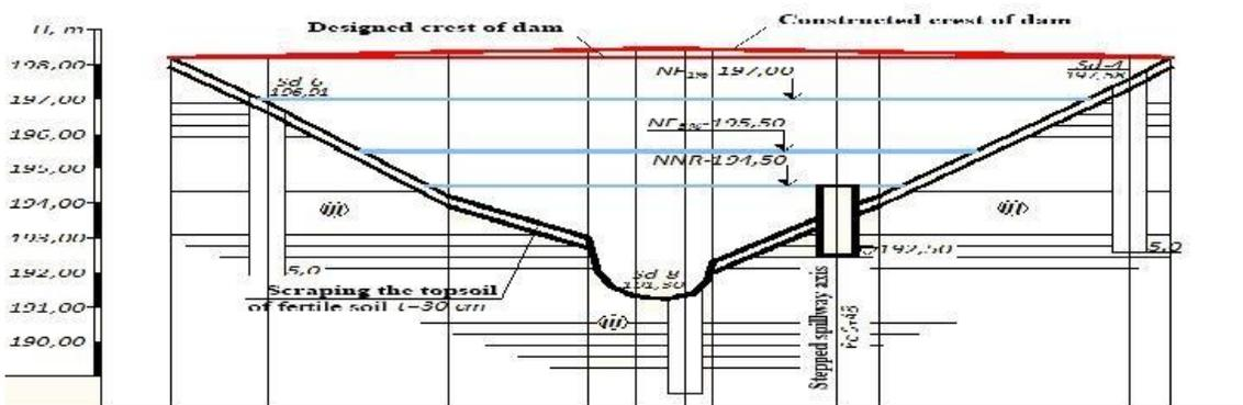
**Figure 5** Longitudinal profile on the dam axis.
