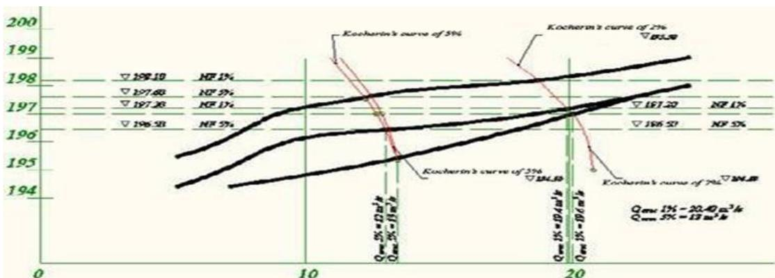
**Figure 4** The scheme to calculate the flow according to Kocherin method.
