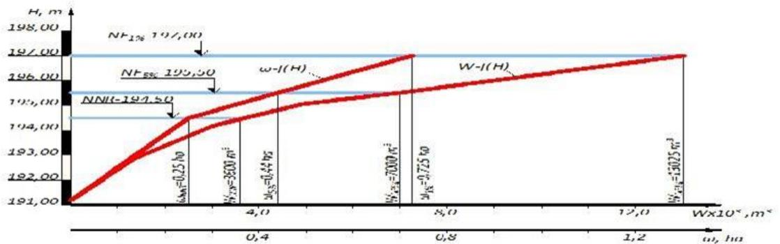
**Figure 3** Bathymetric feature of the pond.
