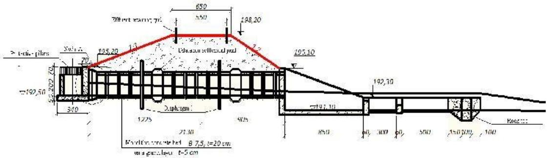
Figure 6 Transverse section of the stepped spillway.
